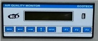
the monitor. Later 1 minute average value are worked out in the logger which can be further averaged and recorded at user defined interval. Logged data can be transferred in computer with the help of pen drive. An USB port is provided for data transfer to computer. The device can be used for routine status monitoring of these pollutants to know the trend of VOC levels prevailing at the monitoring site which are getting influenced
